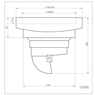
High quality chrome floor grate. Featuring ABS plastic fitting to prevent odours, insects, and suds rising from the floor drainage. Removable for cleaning and maintenance purposes.
