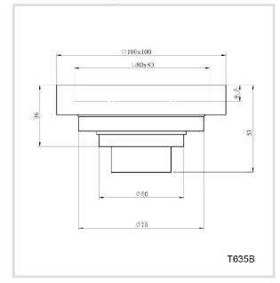
High quality chrome floor grate. Featuring a brass fitting to prevent odours, insects, and suds rising from the floor drainage. Removable for cleaning and maintenance purposes.
